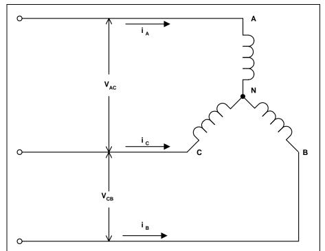
Figure 1 – Measuring power in a 3 wire, 3-phase load using 2 current and 2 voltage waveforms
