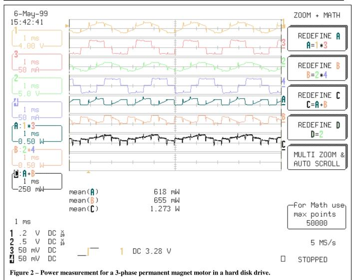
waveform. In this example the average power of traces A, B, and C is being read using the parameter and appear below the waveform display. The total power was measured as 1.273 Watts.
